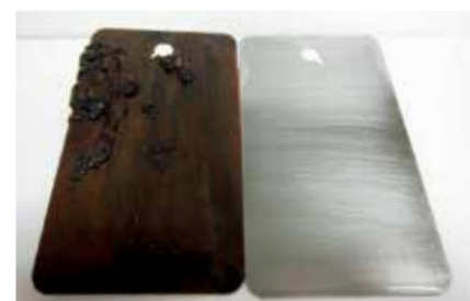
On left; submerged in untreated water (60 ppm Cl - , 300 ppm CaCO 3 ), on right; submerged in AxxaVis HST-10 treated water.
