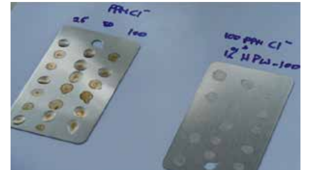
Panel on left cleaned with tap water, panel on right cleaned in a solution of AxxaClean HPW-100.
